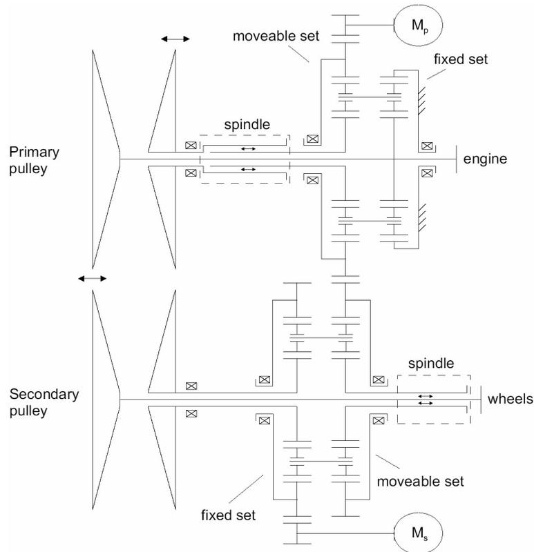
Figure 4: Schematic representation of the servo-electromechanical actuation system.
