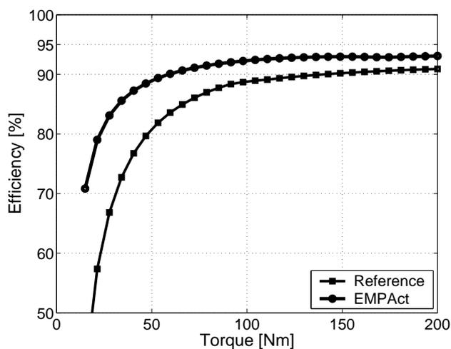
Figure 7: Transmission efficiency comparison for the Reference transmission and the transmission equipped with EMPAct system and variator slip control.
