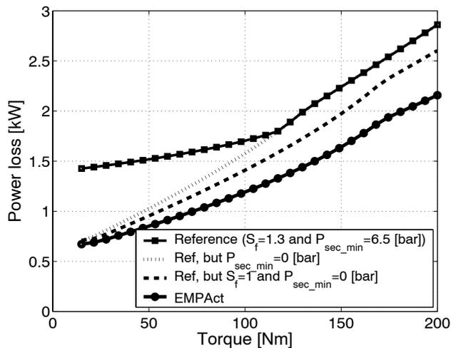
Figure 6: Loss reduction by various measures in comparison to the Reference transmission.
