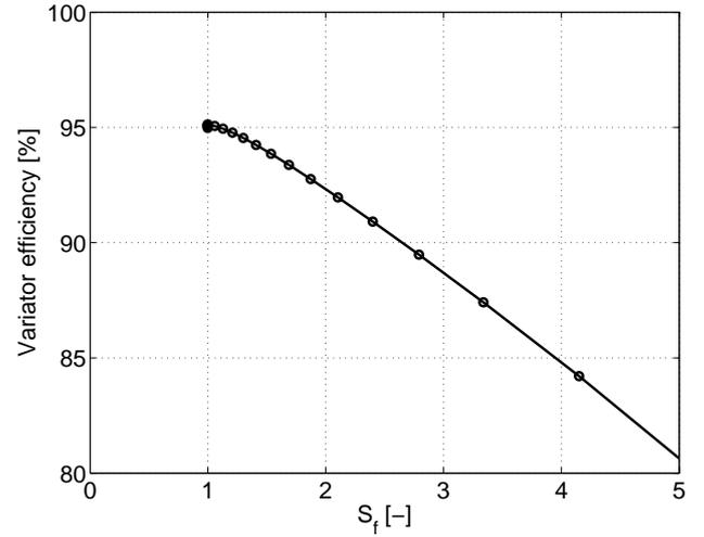
Figure 2: Efficiency versus safety (over-drive, 1500 [rpm]).
