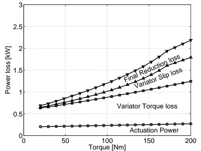
Figure 5: Loss breakdown of transmission with EMPAct system and variator slip control (over-drive, 1500 [rpm]).
