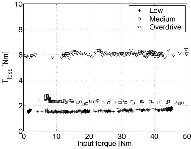
Figure 1: Typical results of  $T_{loss}$  measurements at three different ratios at secondary clamping force of 8 [kN] and 225 [rad/sec] input speed.
