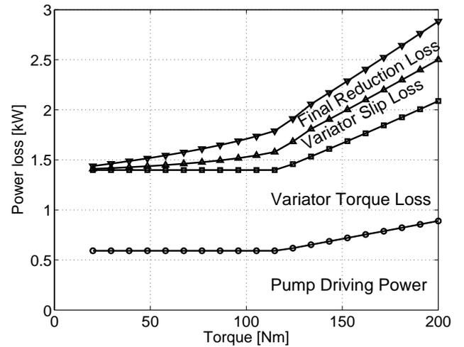
Figure 3: Loss breakdown of reference transmission (over-drive, 1500 [rpm]).
