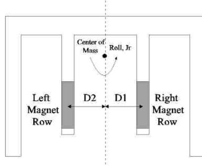
Figure 3: Sled geometry and roll definition
