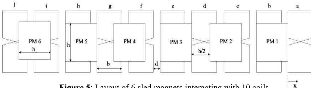
Figure 5: Layout of 6 sled magnets interacting with 10 coils
