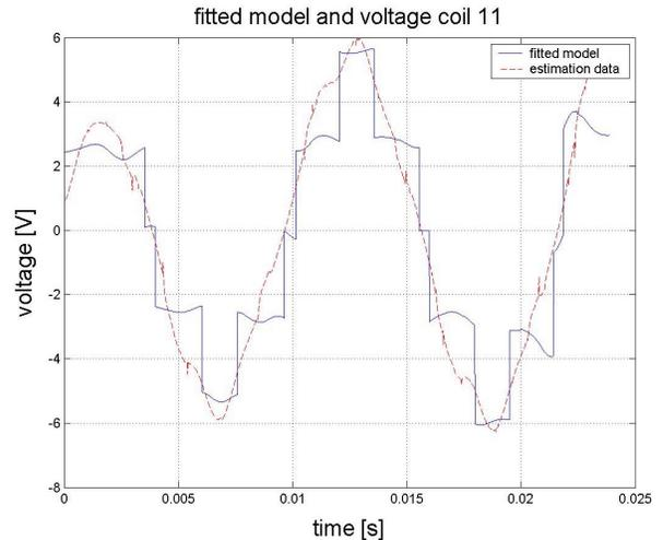
**Figure 11.** Measured voltage vs. simulated voltage (parameter extraction set)
