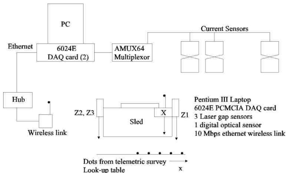
Figure 10: System ID experiment- Estimation of model parameters and model validation
