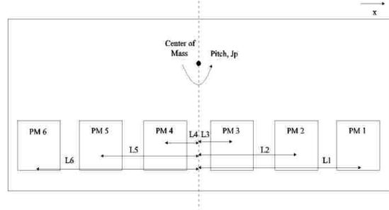
Figure 2: Sled geometry and pitch definition
