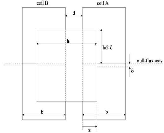
**Figure 1:** Interaction of one magnet with 2 coils
