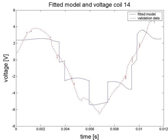
**Figure 12.** Measured voltage vs. simulated voltage (validation set)
