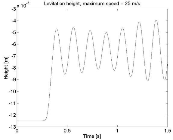
**Figure 7:** Levitation ( $z$ ) respect to null-flux axis
