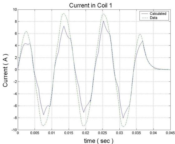
**Figure 13.** Measured current in levitation coil 1 vs. simulated current
